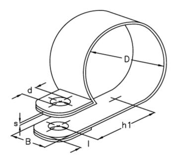
$\begin{array}{ll} d & = 6.4 \\ \text{Diameter D} = 28 \\ \text{h1} & = 23.7 \\ \text{I} & = 6.0 \\ \text{s} & = 0.6 \\ \text{Width B} & = 15 \\ \end{array}$
